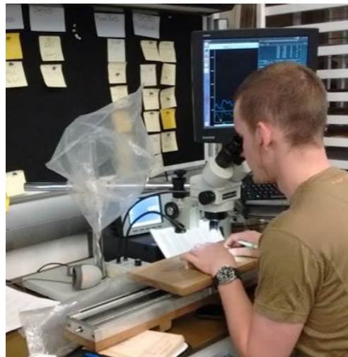
Figure 12. Computer-assisted tree-ring measuring system with microscope.
